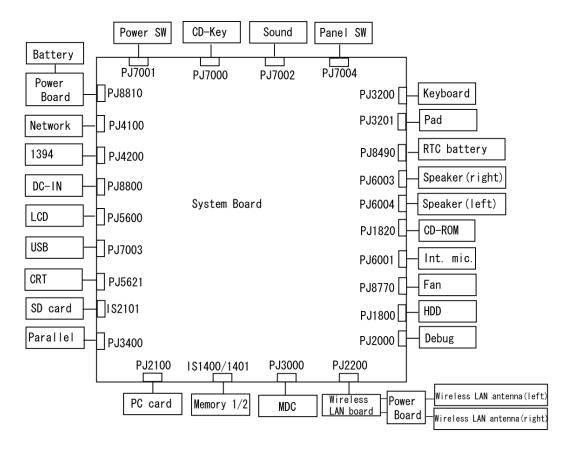
Figure 1-2 System unit configuration
